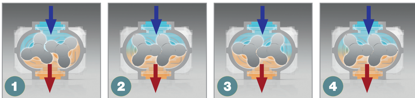
IMAGE 1: Pressure increasing - the images show the cross-section flow chamber of KAESER's rotary lobe blower block.
