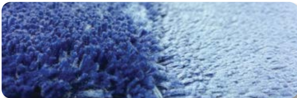
Shown is pile cloth media in its natural state (left) and its conditioned state (right).
