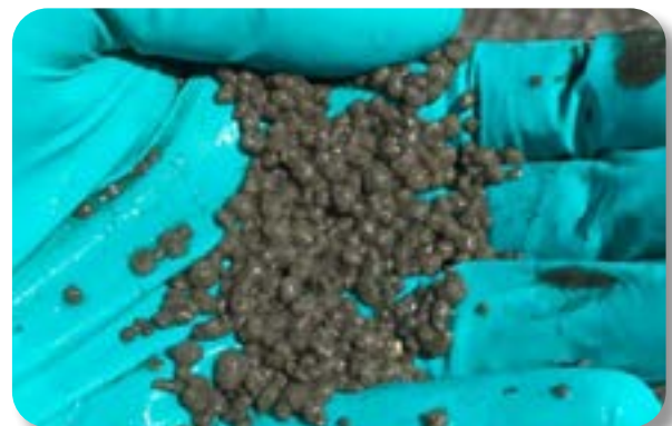
Granule sample following sieve testing at the AquaNereda® demonstration facility, Rockford, IL
