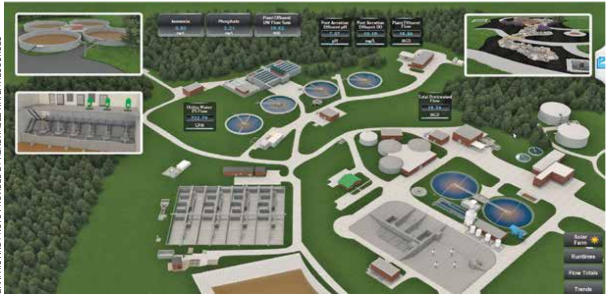
The Wonderware interface (AVEVA) displays one of the utility's eight water resource recovery facilities, now equipped with remote alarm notification supplied and integrated by WIN-911 and MR Systems.
