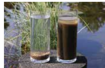
SVI 30 comparison of aerobic granular sludge (left) and conventional activated sludge (right)
